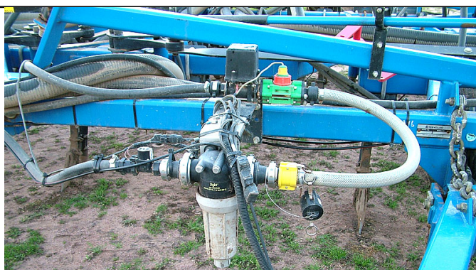
Above: Electric ball valve, low rate flow meter and secondary filtration system mounted off the front of the bar for easy flushing. Ball valve is controlled by a Farmscan Primo 400 spray rate controller. From here product is distributed to the manifolds.
