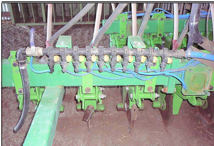
A closer look at the Kirkwood's liquid distribution system and placement on their Walker disc bar.
