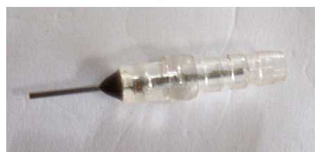
Needle and Luhr in assembly (dispensing needle assembly)
