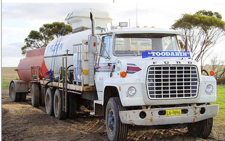
Loui – Our liquid transfer truck. We mix the traces in as we load. Stainless steel tanker and 10,000L tank on truck with 1000L shuttles of sulphates in front.
