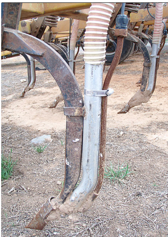
Hydraulic tube mounted on the back of the seed delivery tube.
