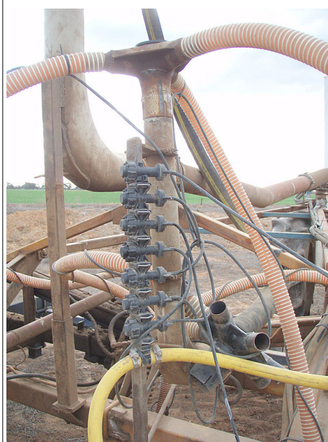
Bank of Wilger nozzle bodies for distribution of the liquids at the air head.
