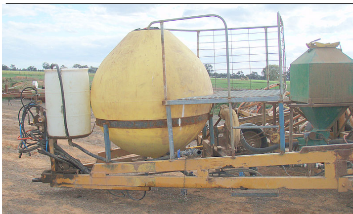
Ryans: Tanks and filling platform (white tank is for flushing, yellow tank is the main Computerspray tank).
