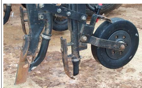
DBS with liquid fertiliser. A very well built and reliable double-shoot knife point seeder.
