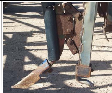
Simple single-shoot knife point with closer plate.
