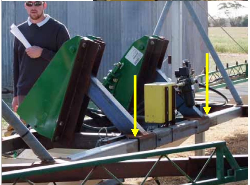
The Eco-Dan controlled shielded sprayer of Leigh Bryan. In photo above, the arrows point to where the spray bar is moved left-right by the Eco-Dan unit. Simple shielded spray modules below that swivel on the bar. Simple and cheap.
