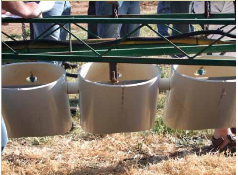
The Eco-Dan controlled shielded sprayer of Leigh Bryan. In photo above, the arrows point to where the spray bar is moved left-right by the Eco-Dan unit. Simple shielded spray modules below that swivel on the bar. Simple and cheap.
